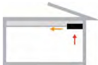
Installation with the ventilation unit partially integrated in the ceiling.
