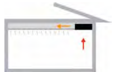
Installation with a diffuse ceiling. The ventilation unit sits above the ceiling with the base plate accessible.
