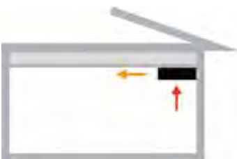
Installation with the ventilation unit under the ceiling.
