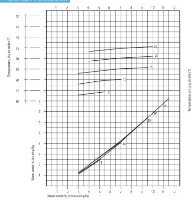
The above capacity diagram is valid for a regenerated air volume of approx. 35 m3/h and a nom. dry air volume of 120 m3/h.
