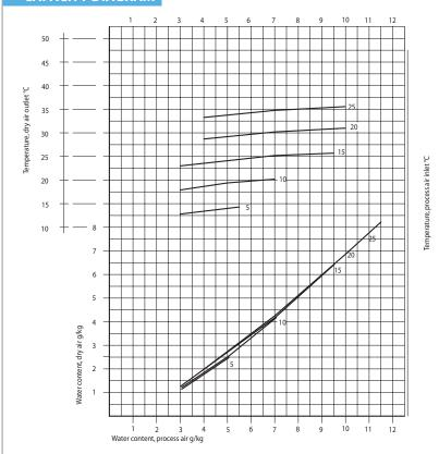
The above capacity diagram is valid for a regenerated air volume of approx. 85 m<sup>3</sup>/h and a nom. dry air volume of 400 m<sup>3</sup>/h.
