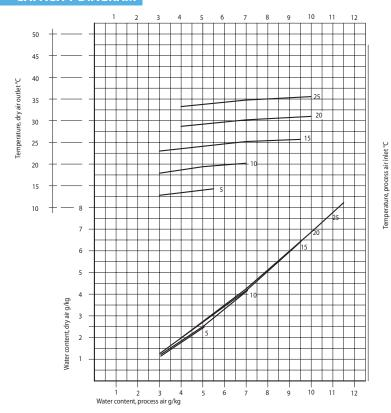
The above capacity diagram is valid for a regenerated air volume of approx. 65 m3/h and a nom. dry air volume of 290 m3/h.
