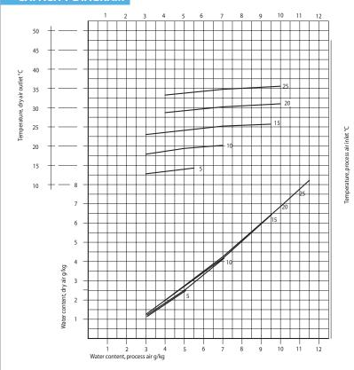
The above capacity diagram is valid for a regenerated air volume of approx. 45 m<sup>3</sup>/h and a nom. dry air volume of 240 m<sup>3</sup>/h.
